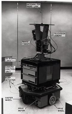
**Shakey the robot** was the first general-purpose mobile robot to be able to reason about its own actions. The project combined research in robotics, computer vision, and natural language processing. Because of this, it was the first project that melded logical reasoning and physical action. Shakey was developed at the Artificial Intelligence
