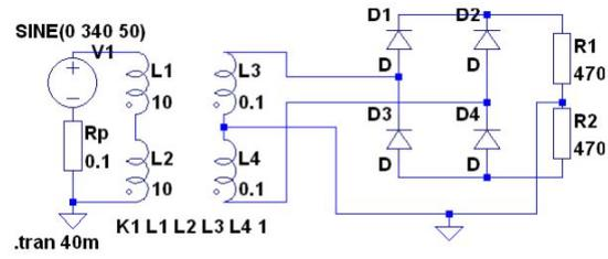
Figure 1: Full wave rectifier with centre tap.
