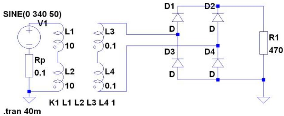
Figure 2: Full wave rectifier with no centre tap .
