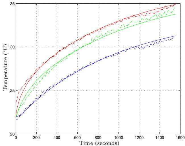
FIG. 6: Results of fitted plot to data. Solid **black** line represents the result from the fitted simulation and dashed lines represent the raw data from the thermocouples. **Red** corresponds to  $x = 0.00$  m, **green** to  $x = 0.075$  m, and **blue** to  $x = 0.15$  m. Heat source is located at  $x = 0.00$  m, as described in Section II 5.
