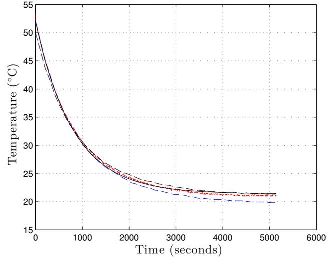
FIG. 5: Results of fitted plot to data. Solid **black** line represents the result from the fitted simulation and dashed lines represent the raw data from the thermocouples. **Red** corresponds to  $x = 0.00\text{m}$ , and **blue** to  $x = 0.15\text{m}$ .
