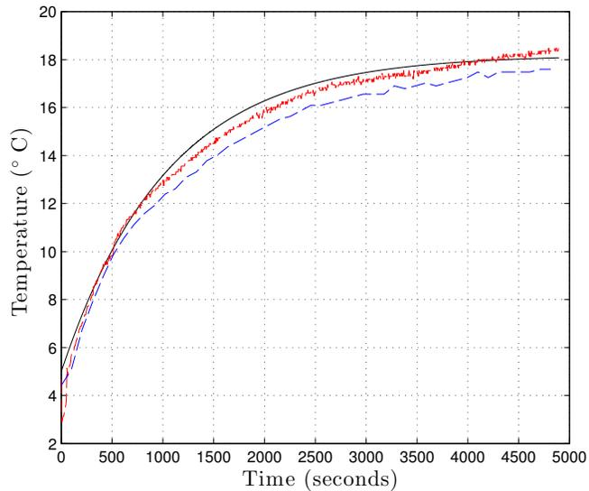
FIG. 2: Results of fitted plot to data. Solid **black** line represents the result from the fitted simulation and dashed lines represent the raw data from the thermocouples. **Red** corresponds to  $x = 0.00$  m, **blue** to  $x = 0.15$  m.
