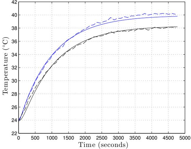
FIG. 4: Results of fitted plot to data. Solid lines represent the simulation and dashed lines represent the raw data. **Blue** to  $x = 0.15\text{m}$  and **black** to  $x = 0.225\text{m}$ . Heat source is located at  $x = 0.00\text{m}$ , as described in Section II 3.
