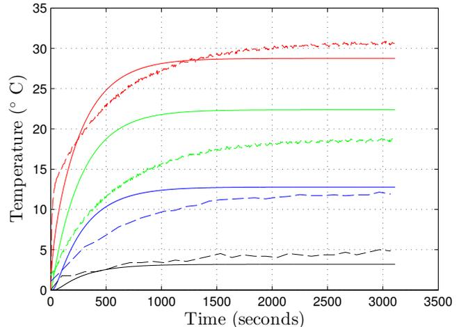
FIG. 1: Results of fitted plot to data. Solid lines represent the simulation and dashed lines represent the raw data. **Red** corresponds to  $x = 0.00$  m, **green** to  $x = 0.075$  m, **blue** to  $x = 0.15$ m and **black** to  $x = 0.225$  m. Heat source is located at  $x = 0.00$  m, as described in Section II 1.
