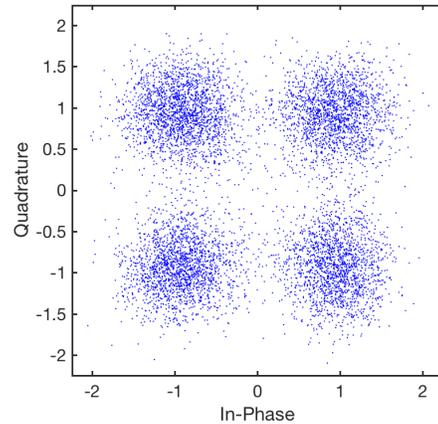
Figure 5: Scatter plot after timing and carrier recovery.
