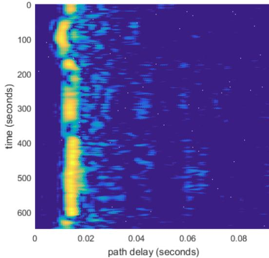
Figure 3: Channel impulse response as a function of time.
