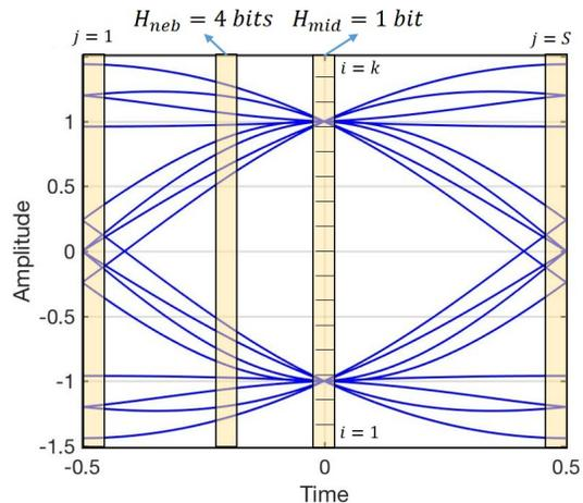
**Figure 1: Eye diagrams of a BPSK signal and its timing phase entropy.**
