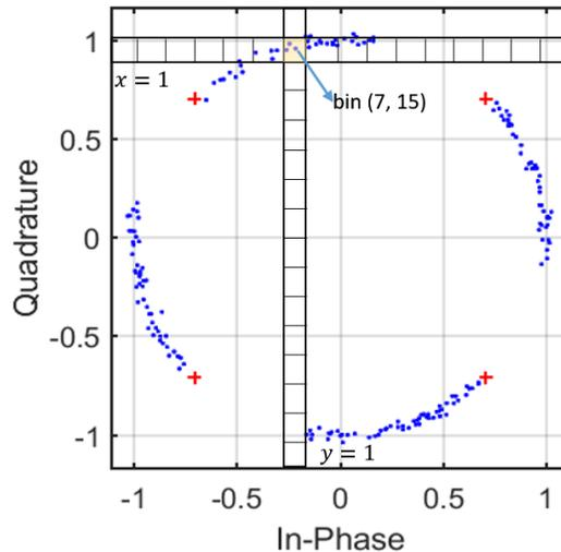
**Figure 2: Constellation diagram of a QPSK signal with carrier frequency offset and its partitions for entropy estimation.**
