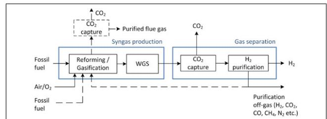
Fig. 2. The route for hydrogen production from fossil fuel sources with  $CO_2$  capture. Solid black lines represent gasification or reformation processing. The dash black lines represents other streams or processing such as methane reformation processing [16].
